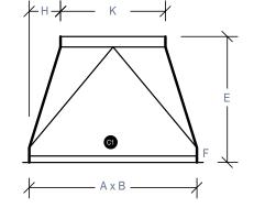
Dimension A = Top Depth Dimension B = Depth Dimension C = Bottom Width Dimension D = Top Extrension Dimension E = Bottom Extension Flange Type C1 Flange Type C2 FT = Flat Top FB = Flat Bottom I = Setting Up/Down/On Top K = Circular Diameter
